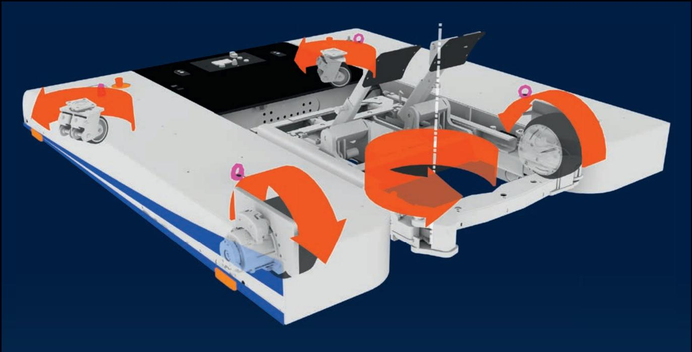
A nosewheel is basically offset in order to remain safely on track during take-off and landing. Due to this, ground position point A is not identical with construction related axis B on the landing gear.
