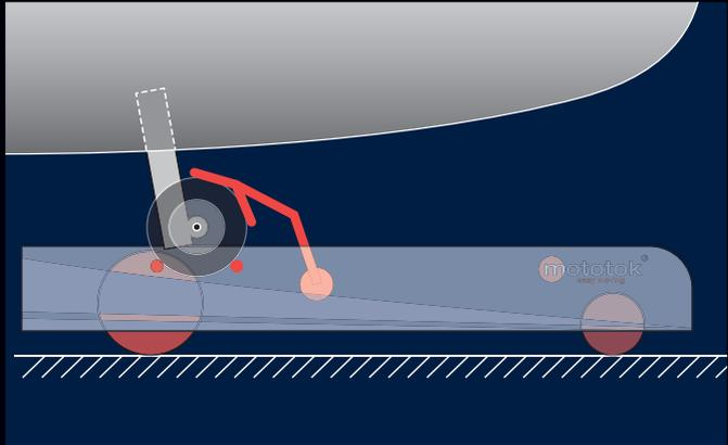
When the nosewheel is raised it is secured by means of the hydro-pneumatically operated wheel securing system.
