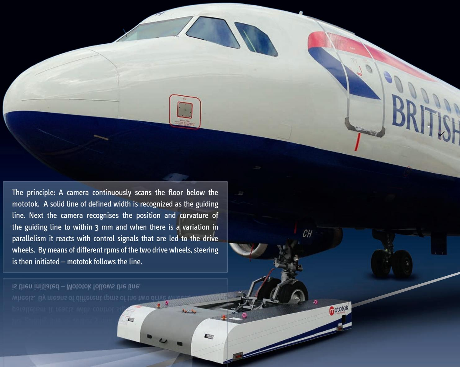
The principle: A camera continuously scans the floor below the mototok. A solid line of defined width is recognized as the guiding line. Next the camera recognises the position and curvature of the guiding line to within 3 mm and when there is a variation in parallelism it reacts with control signals that are led to the drive wheels. By means of different rpms of the two drive wheels, steering is then initiated – mototok follows the line.
